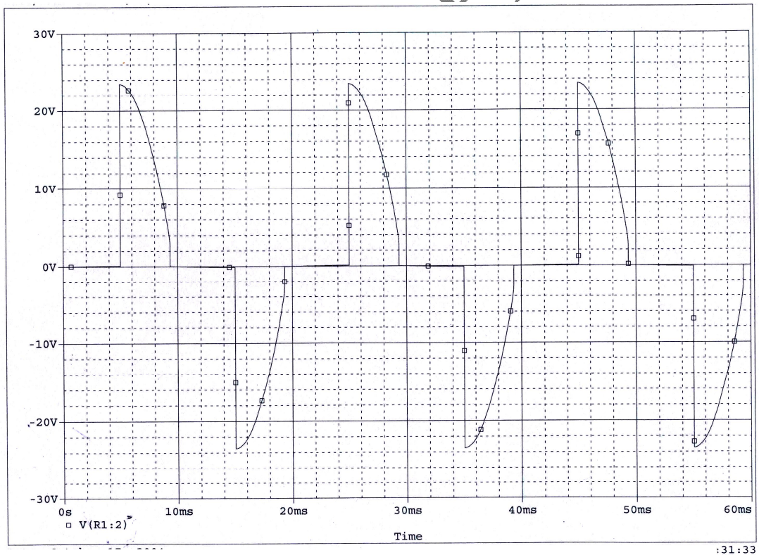
Fig.9 Simulated diagram of single phase AC voltage controller using ORCAD software.
